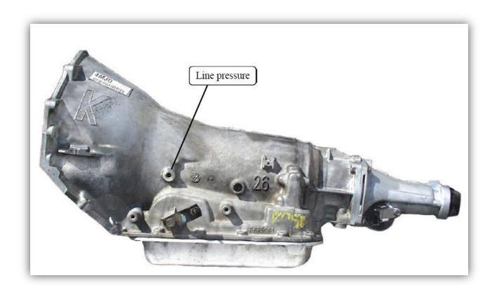
Note: 1998 and later C & K trucks and G vans use a deep pan and filter assembly. If the early shallow filter is installed it will fall off causing low pressures and slippage. Check clearance between pan and filter. The pan is what retains the filter.
